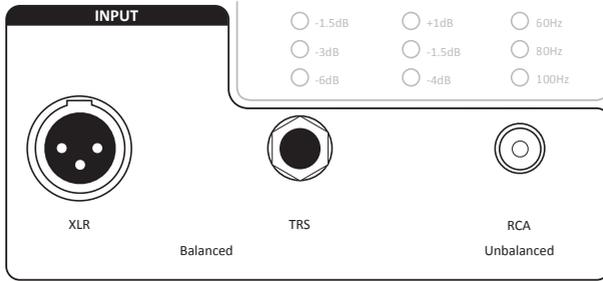
**Line-level Inputs.** The R65/R80 provides a choice of three inputs: two balanced (XLR and 1/4" TRS) and one unbalanced (RCA). These inputs accept a line-level signal from your audio source and feed that signal to the monitor's built-in power amplifiers. When both balanced connections are in use, the TRS input supersedes the XLR input.
