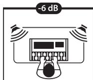
If the monitors are close to the corners of the room, start by setting the Acoustic Space switch to -6 dB, which provides the most bass attenuation.
