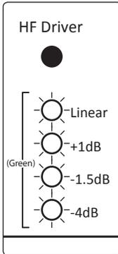
When Energy Conservation mode is active, all four HF Driver LEDs will illuminate green.
