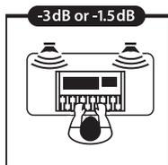
If the monitors are close to the back wall, try setting the Acoustic Space switch to -3 dB or -1.5 dB for less attenuation.
